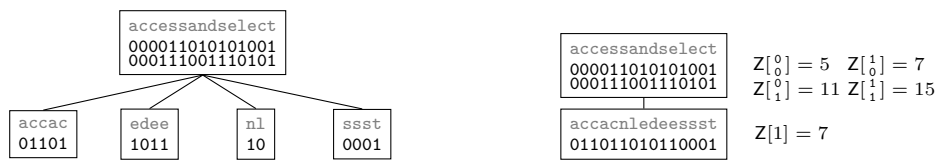
■ Figure 2 4-ary wavelet tree (left) and a 4-ary wavelet matrix (right) for the text accessandselect over the alphabet \{a (000)_2, c (001)_2, d (010)_2, e (011)_2, l (100)_2, n (101)_2, s (110)_2, t (111)_2\} (bit representation of the characters is given in gray), i.e., the same input text as in Figure 1.
